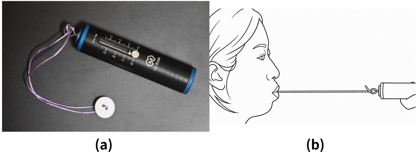
Figure 4. Lip closing strength measurement with the Lip Scale (ROMT Company, Namyangju, Republic of Korea): (a) Lip Scale gauge and its measurement button, connected by a cord; (b) measurement with the button placed in the labial vestibule. The gauge is pulled horizontally, parallel to the floor, until the button is drawn out between the lips, and the reading at that moment is recorded as the lip closing strength in kilograms.
